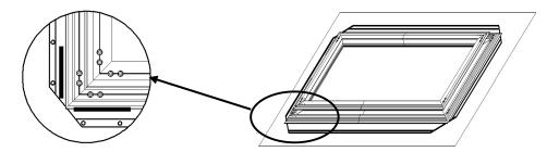
**Step 10:** With one end of the spring and secure inside the groove of the frame, use the *spring hook (d)* to attach the spring to the hole located on the screen material's outer edge in the following order.
