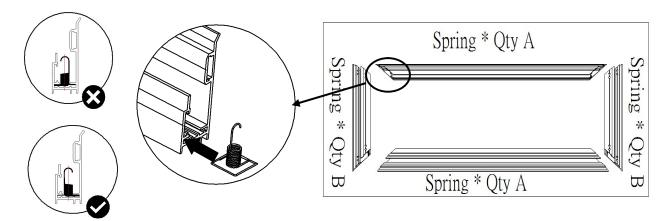
Note: The springs are pre-installed into the grooves of the frame.
