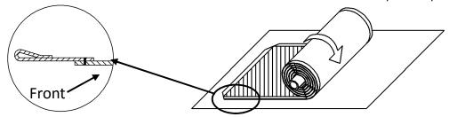
**Step 9:** Carefully and gently place the assembled frame on top of the screen material. Make sure to not allow the angle edge of the frame to come in direct cotnact with the screen material to avoid puncturing it.
