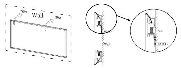
Step 16: With the frame slightly tilted outward; connect the bottom brackets onto the bottom groove of the frame. Then secure them by screwing onto the wall.
