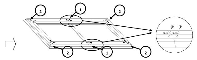
Step 13: Install the angle cover(j) on each corner of the frame and install the LED light strip to hold down the angle cover. Then insert the LED light clip (I) to hold the LED light strip in place.
