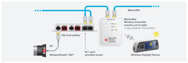
Answer Sure the mounting location does not enable building and glazing features like overhangs, mullions, louvers, or frit to obstruct or cast shadows on the sensor's field of view.
